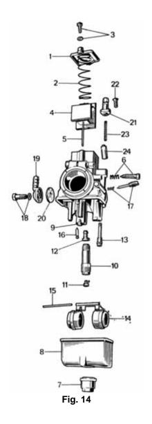
After the carburetor has been stripped and all parts cleaned with an air jet, it is a good practice to inspect and clean the fuel filters and line from the tank.
